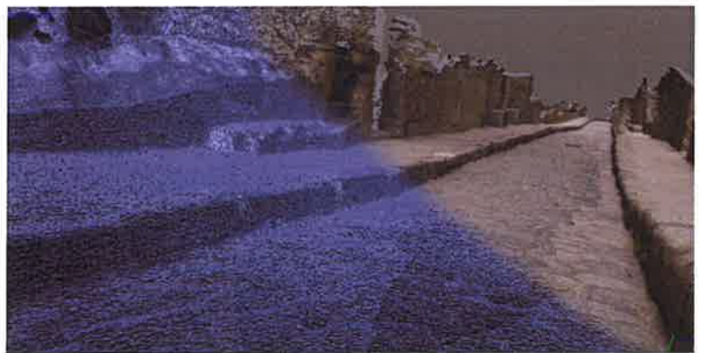
Fig 26. Resulting 3D mesh and overlaying point cloud with visual information preserving color as produced by Agisoft Photoscan.
